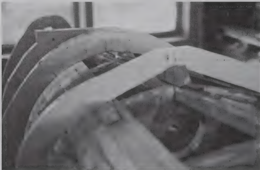
The clamping system which avoids nails and staples.
