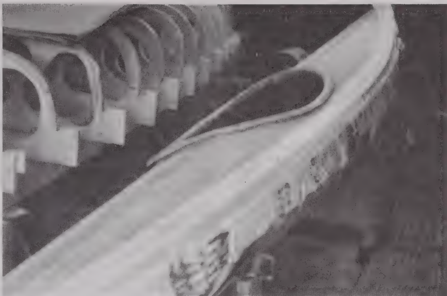
Top being fiberglassed on, notice the paper taped to the side to control runs on the hull.
