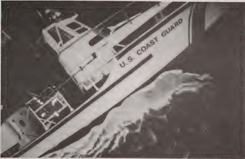
U.S. Coast Guard 44300 was a prototype of a new self-bailing self-righting rescue vessel. Built in 1962 it was positioned at this unusual angle to demonstrate an actual life saving mission. 44300 can be seen from outside the museum through huge windows.
