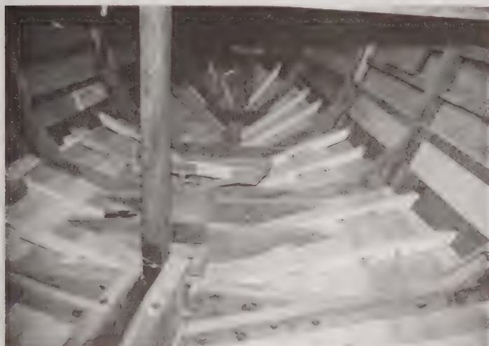
Interior view showing rugged framing. Intermediate frames are Douglas fir.
