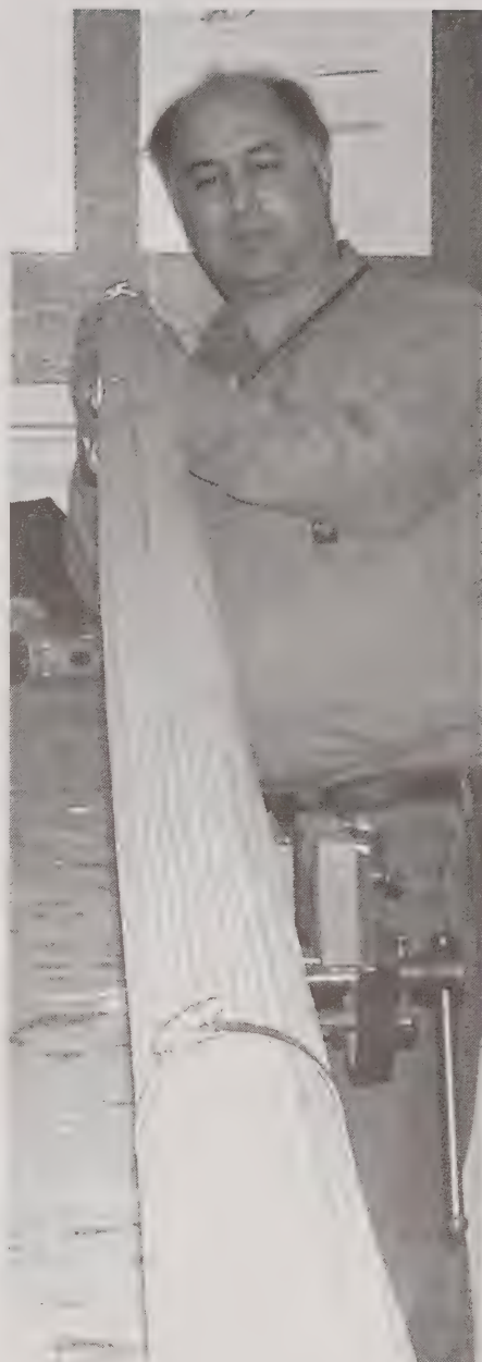
Tom checks the alignment of the dry fit spar as pipe clamps are applied.
