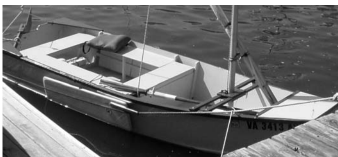
This bright blue flat bottom skiff was rigged with a big aluminum standing lug rig. The owner (my apologies for not noting his name) told me that because the hull was dead flat and wide at the stern it kinda dragged a lot of water along at speed, but still...
