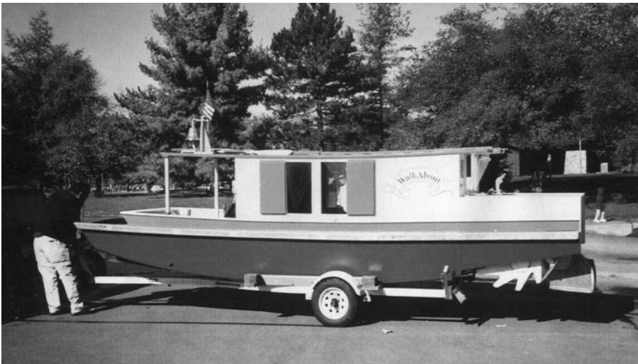
Trailer view shows the rocker of the bottom profile and the raked blades of the sternwheel.
