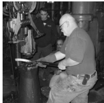
A flowing workpiece starting to take shape as a caulking iron in one of Ray's power hammers.
