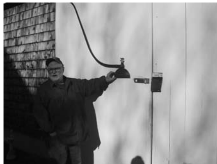
The latch on the doors to Ray's shop is one of his creations, a two man caulking iron for use on deck seams.
