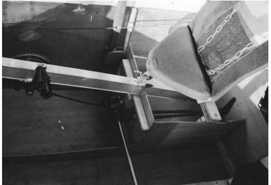
To speed up getting afloat, the seat, pedals, and some other components from a recumbent bike were used. Somewhat different from the design, but effective enough.
