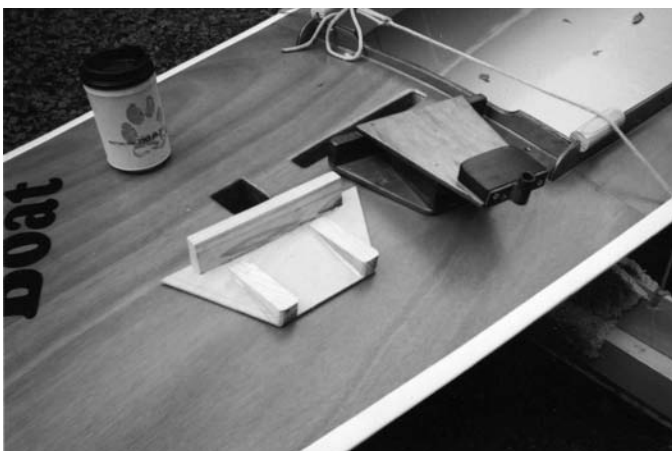
At the oars in the solo rowing station. Outrigger and wedge sitting on forward deck.
