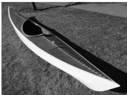
Widgeon Kids Kayak , 14'x24" marine plywood stitch & glue construction, fg cloth exterior, diamond maple wood onlay. Hull painted white. $2,000.
