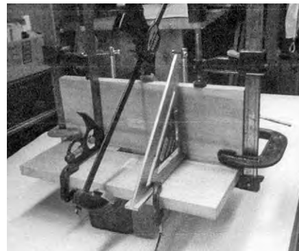
Glued and clamped. The upright piece needs to be exactly square to the base.
