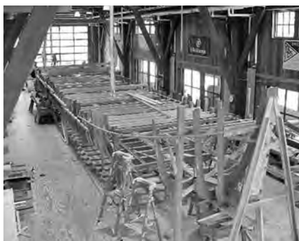
Most of the frames are in and also the cants at the bow.
