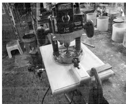
The adjustable guide blocks limit the travel of the router.
