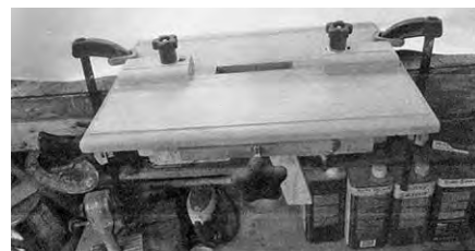
The finished jig clamped to the work bench, ready to cut the first mortise.
