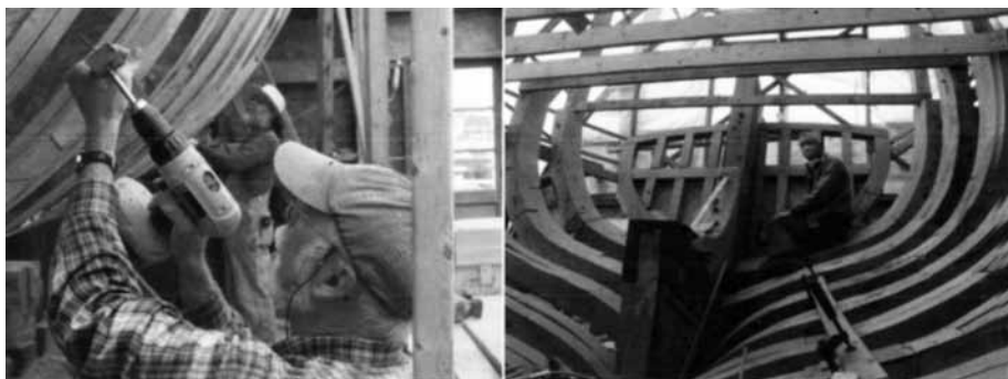
Dr. Dan Wood, with assistance from Tim Teague, sets the fairing batten. Dana Ambrose fairing high on the aft frames with dust mask and hearing protection, safety first!
