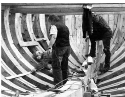
Fairing finesse, Dana applies a batten to the forward portside bilge clamp footprint while Gail Smith and Jim Parmentier stand by for the next high/low spot to work.
