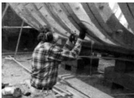
Jim Parmentier (left) checks the fair of the bilge clamp footprint with a batten. Working with shims and epoxy (center), Les Perry fairs the outside hull. Fairing often requires the removal of legacy screws before applying the plank. (Right) Jim employs one of the many forms of removing screws, a large pair of vise grips and some considerable brute force. Some were placed in green wood and are nearly impossible to extract.
