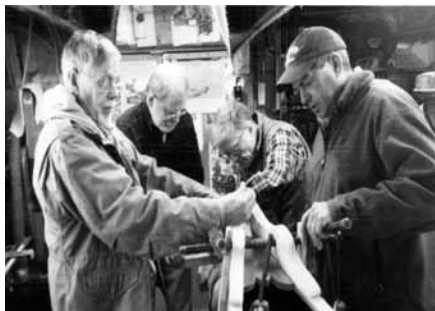
Ken Turner, Mike Clarke, Steve Lapey and John Fitzgerald working the clamps to get one of the outside stems into position.
