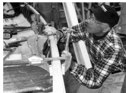
Here we see Jeff Morrill swinging the left handed hammer driving in one of the copper nails.
