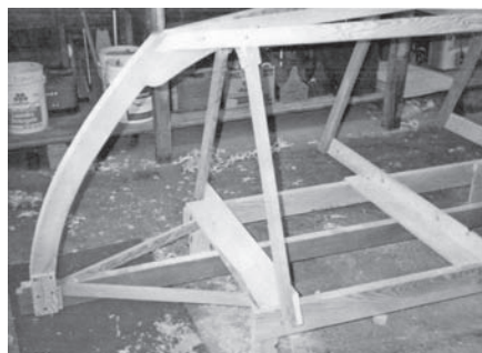
Simple but solid construction setup on ladder frame jog showing stem and forward elements.
