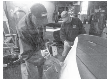
Ed Rothman and Ted Stanton finish priming Lisa's topsides prior to flipping her over.
