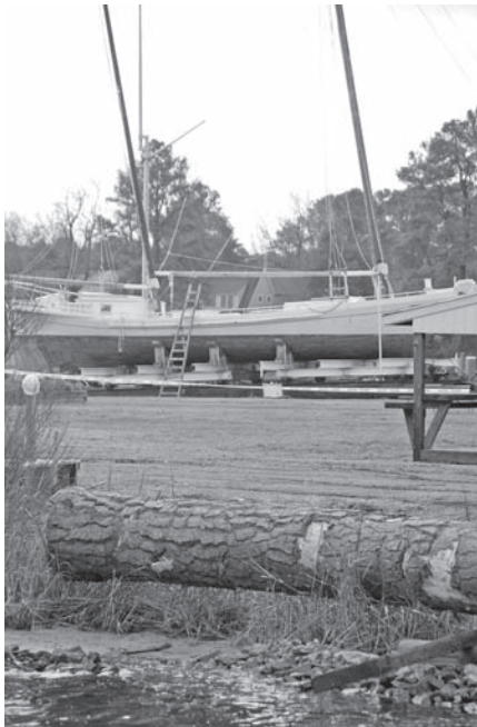
The 1889 log bottom bugeye Edna E. Lockwood , as seen at the Chesapeake Bay Maritime Museum in St Michaels, Maryland, with one of the loblolly pine logs that will be used for her log hull restoration in the foreground.
