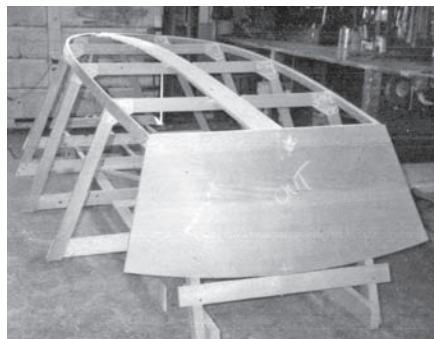
More construction showing frames and transom set up on ladder frame.
