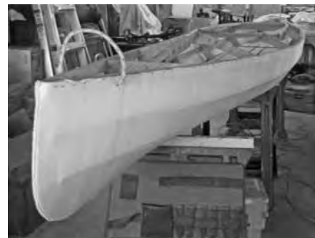
Hull stapled, stem and stern sewn, fabric trimmed.
