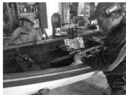
Andy Strode and Steve Tulka repairing the thole pin sockets on Ellysea , the Boston Whitehall.
