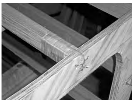
Deck beam lashed to second former.
