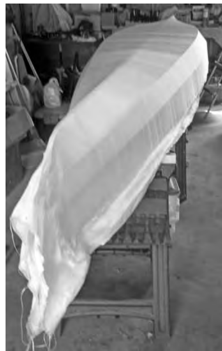
Fabric draped and stapled, clamps at ends removed.
