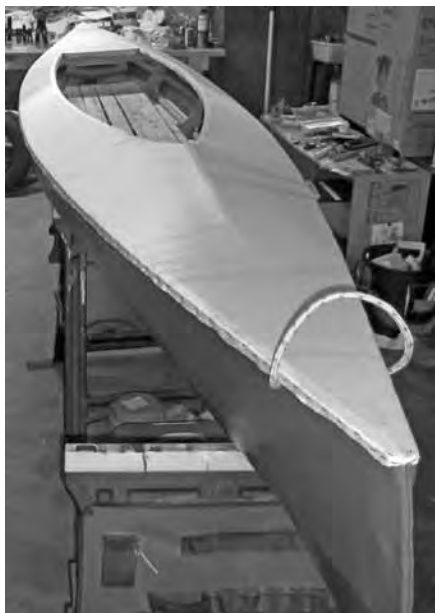
Deck attached and trimmed
