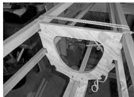
Keel and gunwales lashed to stem, stringers being bent before trimming and lashing.
