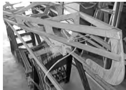
Keel and gunwales lashed to stem, stringers being bent before trimming and lashing.
