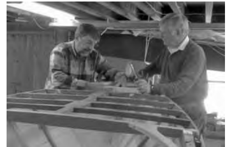
Stewart Close and Pierce Hance are securing another segment in the bow of the Herreshoff 12 1/2 sloop.
