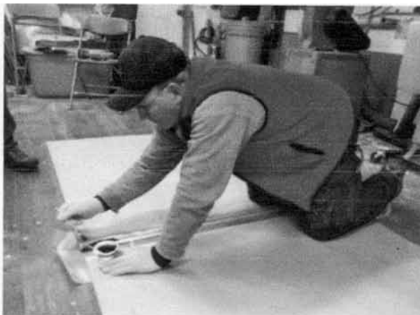
Dan Nelson gluing scarf for Dory bottom.
