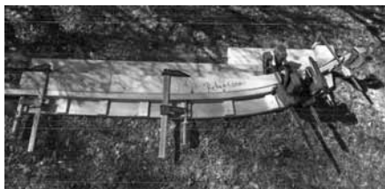
The same gunwale bending form that we used last year for the Robertson needed just a few changes to match the curve of the Kennebec.
