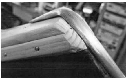
Rail caps, outwale and stem band all have to line up just right at the tips.
