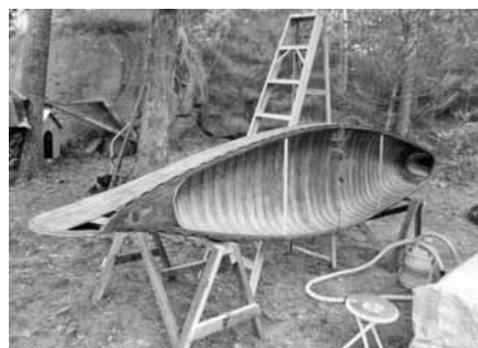
Lawton found that it was easier to just concentrate on the bottom of the canoe first and then tip it up onto one side and then the other side. This kept the stripper flat on the painted surface in a thicker coat, allowing it to do its job better. It was still a long, messy task, but rewarding when it was done.
