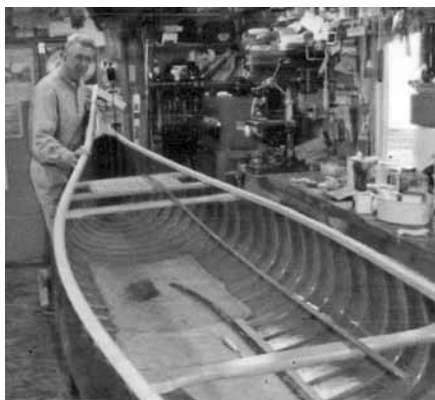
This rail cap is almost completely nailed in place, the ends have been left loose so we will be able to trim them and make the joint when the other cap is in place.
