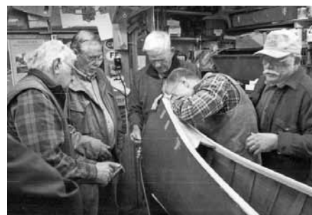
Lawton Gaines, Ken Turner, Roger Andrews, Steve Lapey and Ed Moses work to line up the rivets for the stem band.
