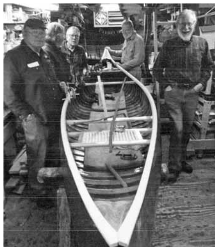
Rail caps in place secured with brass escutcheon pins. From left to right, Stuart Fall, Lawton Gaines, Steve Lapey. Mike Clarke and Bill Clements.
