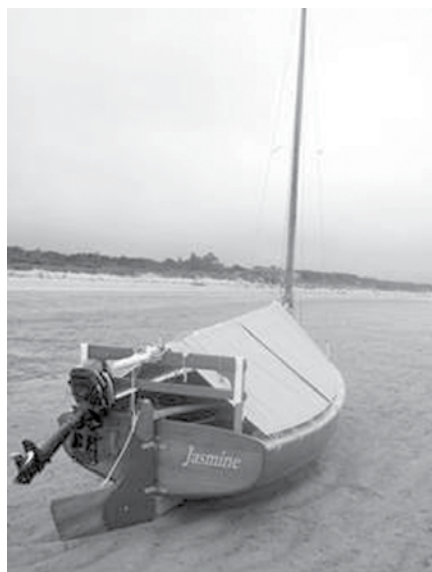
15' Joel White Catboat , $7,500, laying Mattapoisett Harbor, near New Bedford, MA. And it's a beauty. Joel White "Marsh Cat" design, 1400lbs displacement, 6'11" beam. Draft w/cb up a scant 9", 2'-8" down. Cold-molded epoxy glued marine plywood hull & decks. Always shedded. Hull built by L. Daniel Fry, Williamsport PA. Lots of unique & handy features, incl a mahogany lazaretto, boom gallows, roomy mahogany seats & folding mast tabernacle by Redd's Pond Boatworks, Marblehead, MA. Incl custom-tailored canvas boom tent by Ocean Tailors, '09, '07 LoadRite trlr (Model 16125076V) upgraded with fast-hinge tongue to fit in shallow garage or shed, Tohatsu 5hp long-shaft motor (model M5BL, SN 10248). Jasmine is thoughtfully rigged in ready-to-sail condition w/ anchor & mahogany chain storage box, custom-mounted compass, handmade wooden cleats, jiffy reefing, retractable rudder & fenders. Guzzler bilge hand pumps installed in lazaretto, with dual port/starboard control valves. Exc cond w/fresh painted bottom & 3 coats of varnish on all bright work, Fall 2014. JOE THOMPSON, (413) 664-4481, x8 100, 15ft-Catboat4sale@gmail.com (9)
