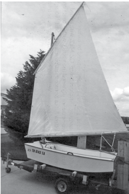
Puddle Duck , $750. Built in 2008, very lightly used & completely restored by owner/builder in 2016. Exc cond; needs nothing. Michael Storer OZ Mk2, w/added side tanks/dagger board. Hull pine exterior plywood (no voids), with 3 coats epoxy plus exterior primer/enamel. Hollow Sitka spruce mast/pine spars. Sail 105sf from Dave Gray Polysail kit; two reef points. Very "yachty" with bright oak trim & boards. All stainless fasteners throughout. Trailer shown available for $150 w/boat. JIM BROWN, Sweetwater TN, (423) 8369058, whitedove0215@yahoo.com. (10)
