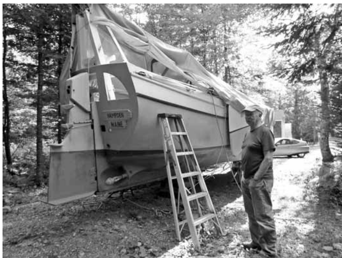
Alert's stern quarter with Stan. Note off center prop, stout end plate on her rudder and that vital ladder up the rudder.
