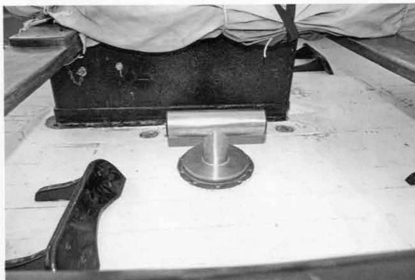
Seen from the starboard gunwale, bows to the right. Stainless steel bilge vents for harbour use only. They are replaced with screw-in Henderson hatch covers before sailing. The stretcher (left) is for the feet of the seated oarsman (right). The intakes of two relieving valves can be seen behind the vent on either side of it. (They are non-return drains to rid the cockpit of water – ten altogether)
