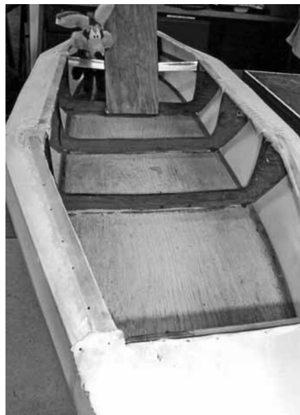
Wylie Coyote inspecting the new Dacron fabric covering.
