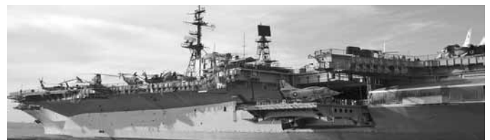
LHD-2 USS Essex , one of the eight ship Wasp Class, at 40,000 tons carrying US Marine Corps helos and jump jets with a well deck below the hangar deck to carry landing craft hauling USMC 70ton tanks etc.
