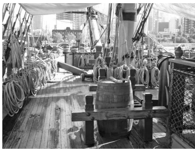
Towards the bow, with the lower end of her foremast, standing and running rigging, lots of lines, all human powered, here on deck, with more high aloft in scary places.
