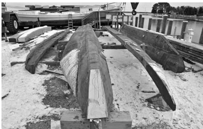
All nine of the loblolly pine logs needed to replace the the hull have been selected and shaped.
