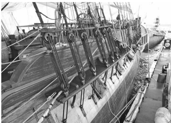
The standing rigging to keep fore and mainmasts standing, a complex system of tendons and bones.
