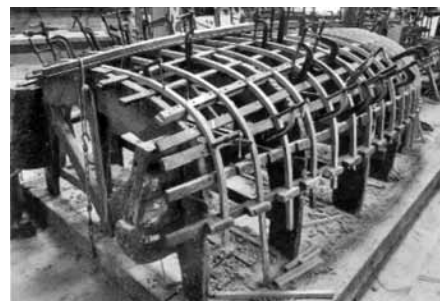
Frames bent on the mold.
