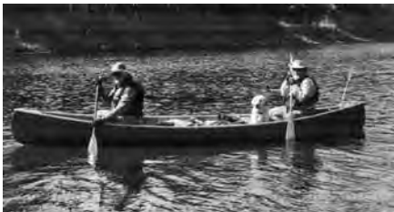
Alan, Finn and Tom in the canoe Tom made. It is 17' long, 38" wide and made of sassafras.
