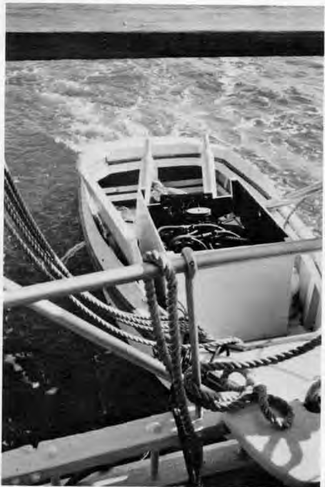
"Martha Lewis" yawl boat. The powerful push-boat is used for leaving the harbor and returning to harbor, and for dredging under power only on Mondays and Tuesdays, by Maryland law, as a conservation measure.
