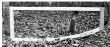
This next picture is essentially the port side frame for the aft section (still needs the outer layer and a few fasteners, but this is the basic shape).
