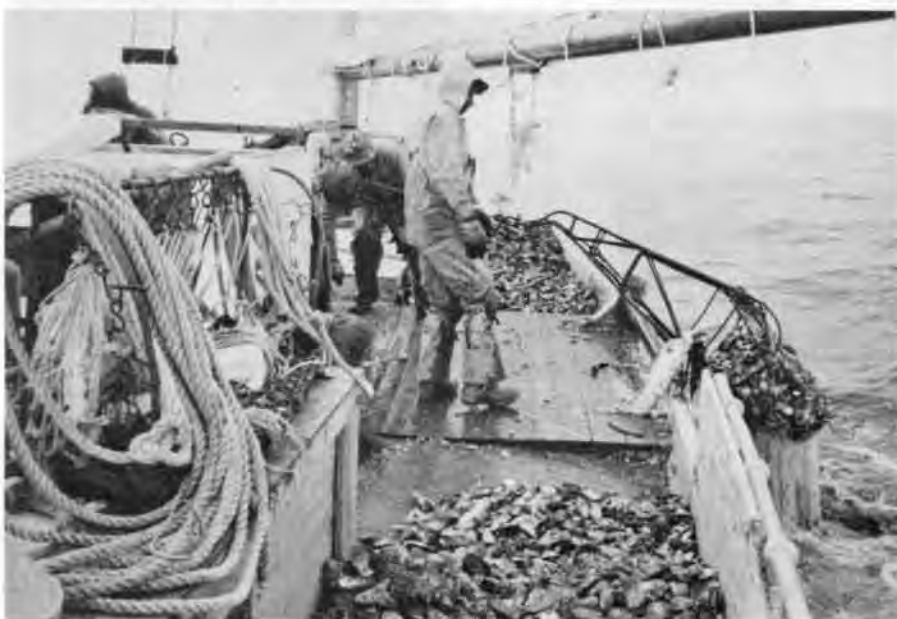
A gasoline engine (the winder) hauls the dredge aboard over the roller. Grabbing the large rings, the crew lift it onto the deck.
